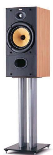
Description 2-way vented-box system Power handling 25W - 120W into 8 ohm on unclipped **Drive units** 1 x 25mm metal dome high-frequency programme 1 x 180mm woven Keylar® cone Dimensions Height: 490mm Width: 236mm bass/midrange Depth: 306mm **Finishes** Cabinet: Cherry or Black Ash Vinyl, Frequency response  $52Hz - 20kHz \pm 3dB$  on reference Grilles: Black cloth Sensitivity 90dB spl (2.83V, 1m) Nominal impedance 8 (min 4.3 )
